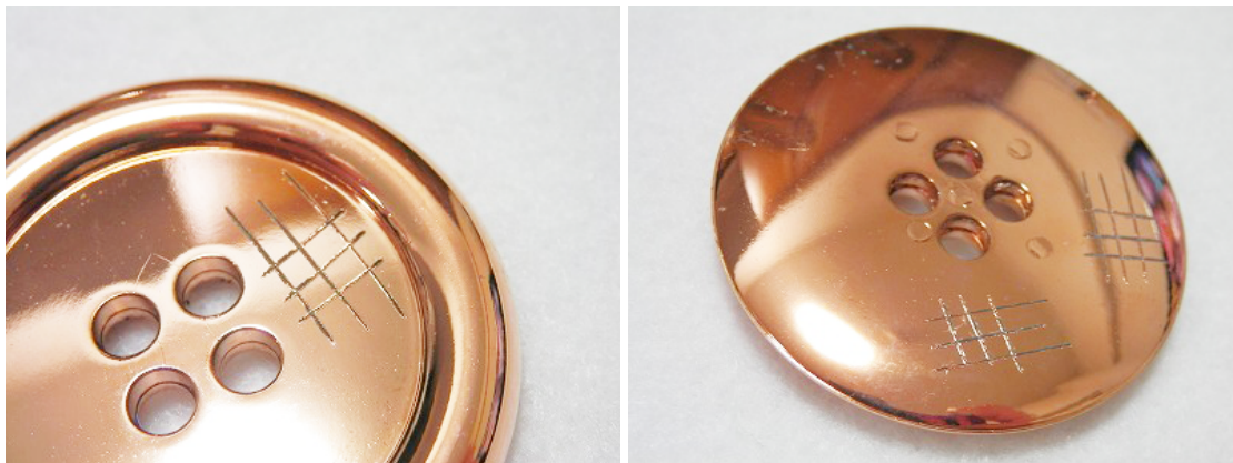
Figure 7 The Copper plated samples were fabricated using a substrate ABS.
